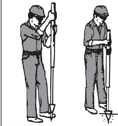
The Pilot Hole Driver is a quick way to prepare the ground when a starter hole is necessary. Follow this procedure:
